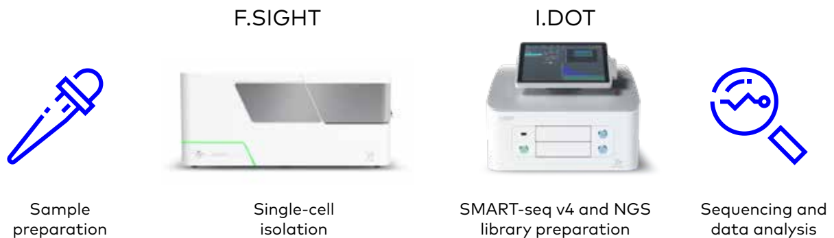
Figure 1. Miniaturized and high-throughput workflow for generating single-cell RNA sequencing libraries. After sample preparation, the f.sight isolates single cells into PCR well plates, which undergo library prep with the I.DOT. The resulting libraries are sequenced and further analyzed.
