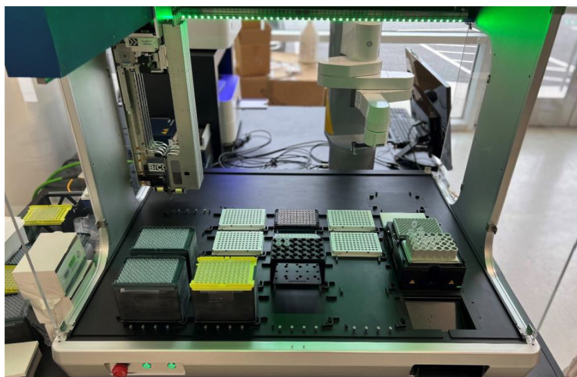
Figure 2. Deck Set up on the automated Liquid Handler for application start-up, with tip storage, reagent plates, shaker and cooling module.
