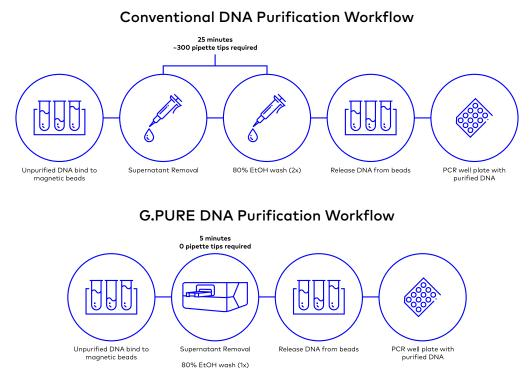
**Figure 1.** The G.PURE provides a fast and automated workflow for bead-based DNA purification. Standard manual bead cleanup workflows are time-consuming and require many pipettes due to the several removals, wash and dispense cycles used to purify the DNA. The G.PURE performs the critical wash steps 5x faster than conventional purification while requiring no pipetting steps.
